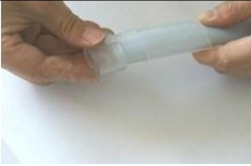
9. Attach End cap to the other end of NEONFLEX
